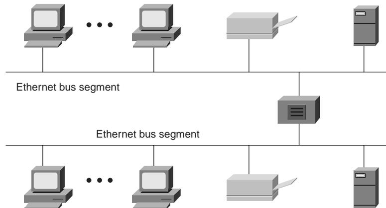
Although new networks are no longer connected in a bus configuration, some older bus-connected networks do still exist and are still useful.
