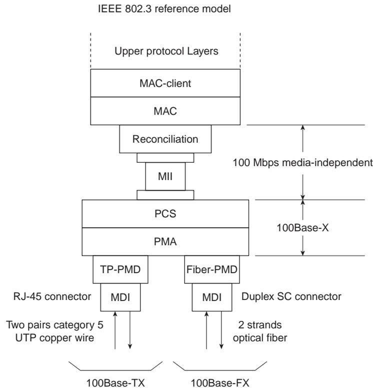
The 100Base-X encoding procedure is based on the earlier FDDI optical fiber physical media-dependent and FDDI/CDDI copper twisted-pair physical media-dependent signaling standards developed by ISO and ANSI. The 100Base-TX physical media-dependent sublayer (TP-PMD) was implemented with CDDI semiconductor transceivers and RJ-45 connectors; the fiber PMD was implemented with FDDI optical transceivers and the Low Cost Fibre Interface Connector (commonly called the duplex SC connector).
