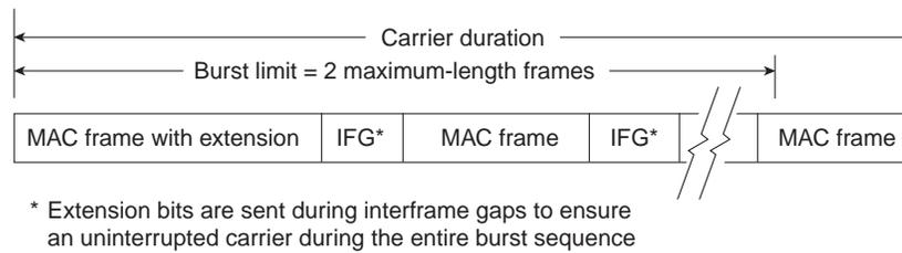
If the length of the first frame is less than the minimum frame length, an extension field is added to extend the frame length to the value indicated in Table 7-1. Subsequent frames in a frame-burst sequence do not need extension fields, and a frame burst may continue as long as the burst limit has not been reached. If the burst limit is reached after a frame transmission has begun, transmission is allowed to continue until that entire frame has been sent.
