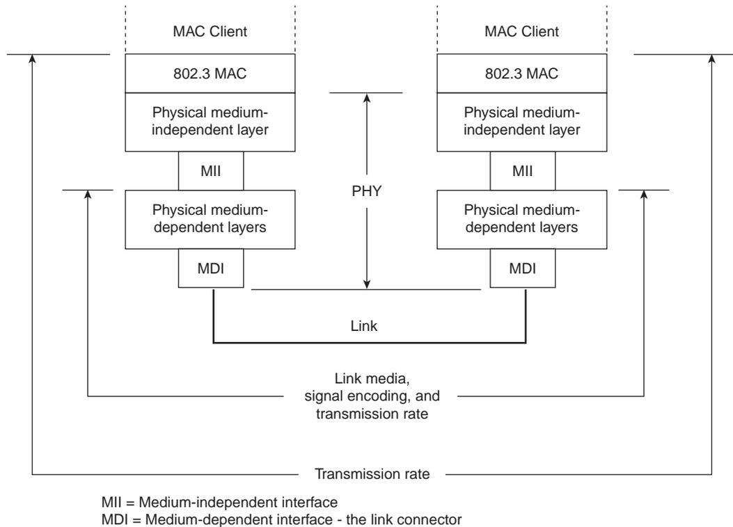
The MAC layer controls the node's access to the network media and is specific to the individual protocol. All IEEE 802.3 MACs must meet the same basic set of logical requirements, regardless of whether they include one or more of the defined optional protocol extensions. The only requirement for basic communication (communication that does not require optional protocol extensions) between two network nodes is that both MACs must support the same transmission rate.
