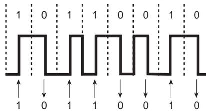
Unfortunately, Manchester encoding introduces some difficult frequency-related problems that make it unsuitable for use at higher data rates. Ethernet versions subsequent to 10Base-T all use different encoding procedures that include some or all of the following techniques:
