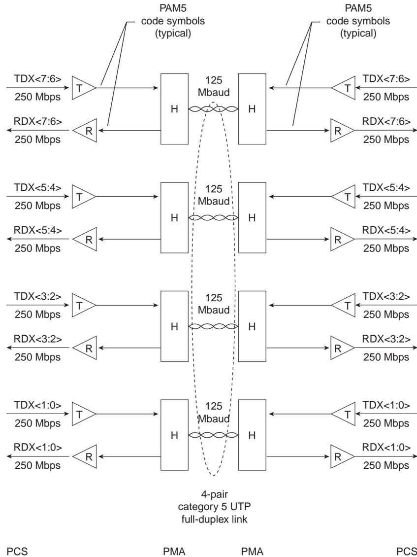
The clock recovery and master/slave loop timing procedures are essentially the same as those used in 100Base-T2 (see Figure 7-24). Which NIC will be master (typically the NIC in a multiport intermediate network node) and which will be slave is determined during autonegotiation.
