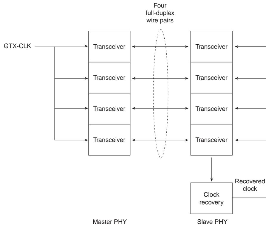
Each transmitted frame is encapsulated with start-of-stream and end-of-stream delimiters, and loop timing is maintained by continuous streams of IDLE symbols sent on each wire pair during interframe gaps. 1000Base-T supports both half-duplex and full-duplex operation.
