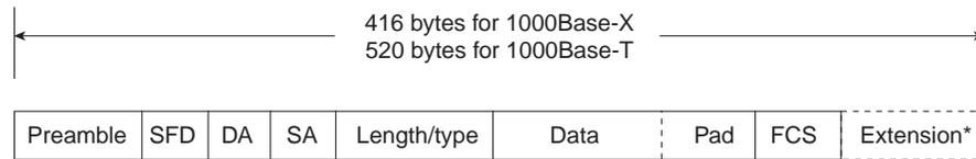
\* The extension field is automatically removed during frame reception
