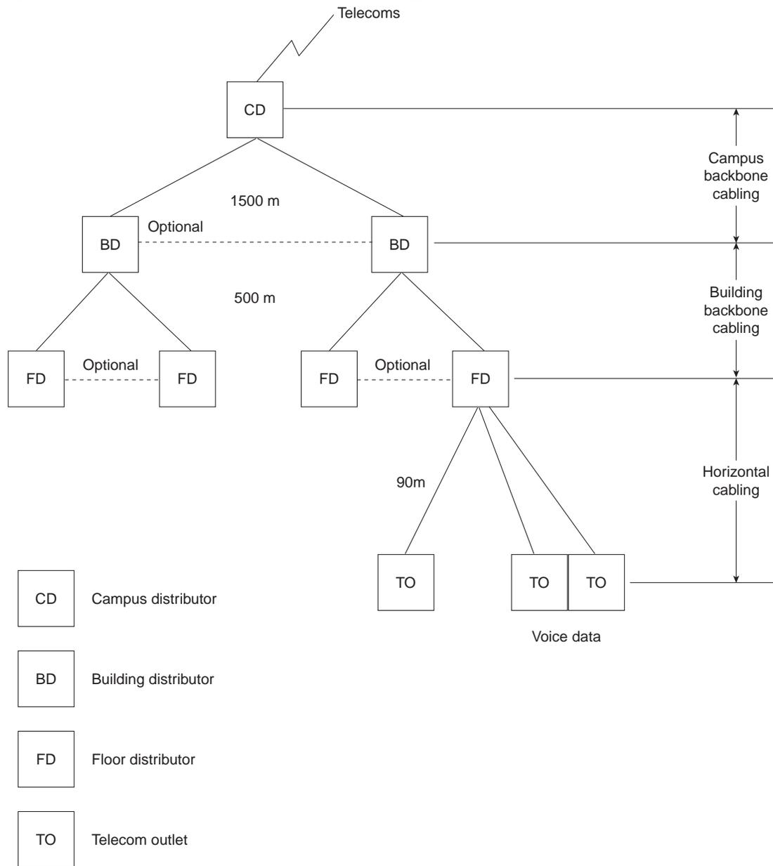
The ISO/IEC 11801 cable model is the network model on which the IEEE 802.3 standards are based:
