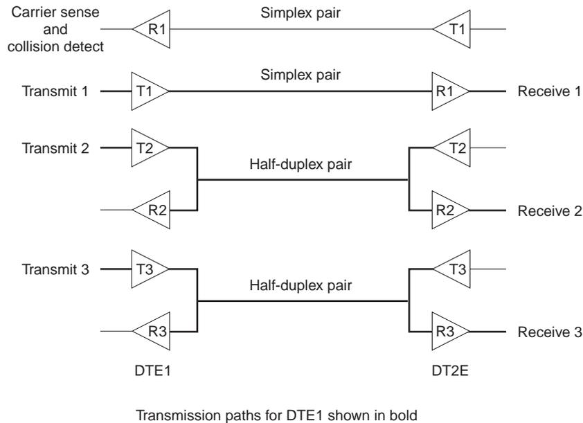
100Base-T4 uses an 8B6T encoding scheme in which each 8-bit binary byte is mapped into a pattern of six ternary (three-level: +1, 0, -1) symbols known as 6T code-groups. Separate 6T code-groups are used for IDLE and for the control code-groups that are necessary for frame transmission. IDLE received on the dedicated receive pair indicates that the link is quiet.
