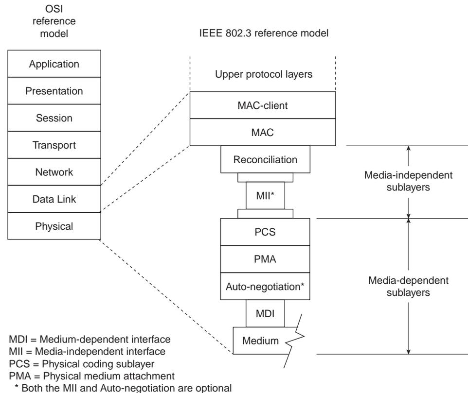
The physical layer for each transmission rate is divided into sublayers that are independent of the particular media type and sublayers that are specific to the media type or signal encoding.
