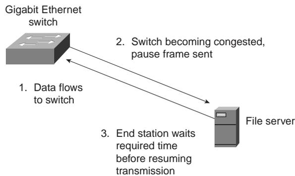
The full-duplex operation and its companion flow control capability are both options for all Ethernet MACs and all transmission rates. Both options are enabled on a link-by-link basis, assuming that the associated physical layers are also capable of supporting full-duplex operation.
