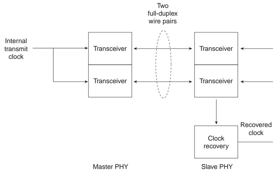
The 100Base-T2 encoding process first scrambles the data frame nibbles to randomize the bit sequence. It then maps the two upper bits and the two lower bits of each nibble into two five-level (+2, +1, 0, -1, -2) pulse amplitude-modulated (PAM5) symbols that are simultaneously transmitted over the two wire pairs (PAM5x5). Different scrambling procedures for master and slave transmissions ensure that the data streams traveling in opposite directions on the same wire pair are uncoordinated.
