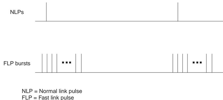
At first glance, it may appear that the autonegotiation process would always select the mode supported by the NIC with the lessor capability, which would be the case if both NICs use the same encoding procedures and link configuration. For example, if both NICs are 100Base-TX but only one supports
