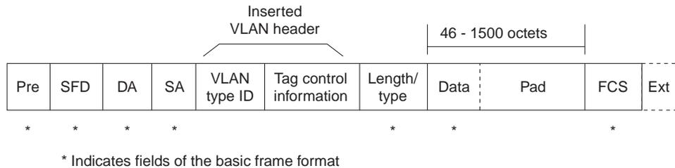
The VLAN header consists of two fields:
