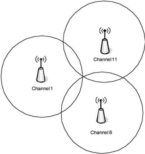
Like the noisy hotel room, it may also be necessary to limit the power output from the access point so that the “noise” from one access point does not impact your neighbors. Careful study of the locale of the wireless network will help you understand what output levels are acceptable.
