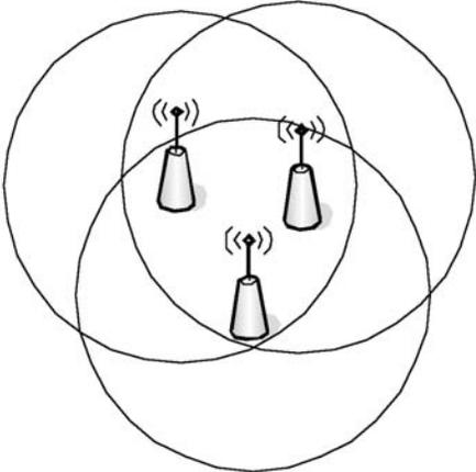
The designers of the 802.11b/g protocols set aside three channels that do not overlap. Channels 1, 6, and 11 are separated by enough space so that they do not get into each other's way when the access points are properly configured. Assigning adjacent access points to different channels—especially 1, 6, or 11—will help reduce the path-sharing problem.
